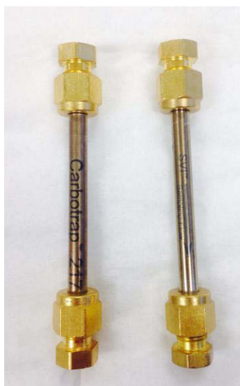
Figure 7. Photograph of Carbotrap ® (left) and SVI ™ (right) TDTs (Photo: Loay Jabre)
