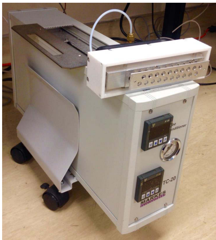
Figure 8. Photograph of the TC-20™ Tube Conditioner, with the tube holder resting on top of the instrument (Photo: Loay Jabre)
