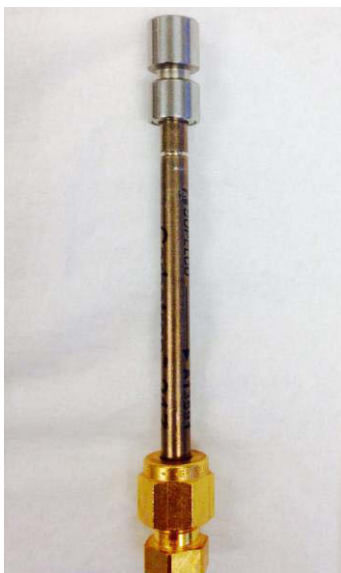
Figure 10. Photograph of a TDT with a DiffLok™ show on the top of the tube (Photo: Loay Jabre).
