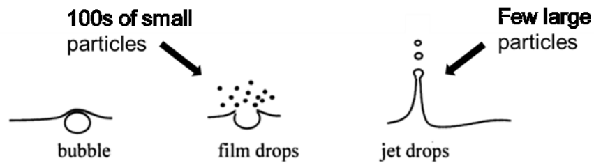
Figure 2.1 The production of droplets from bubble bursting at the surface of the ocean. The differences in the production mechanisms are shown, as well as an indication of the differences in the number of droplets produces. Adapted from (Resch et al., 1986).
