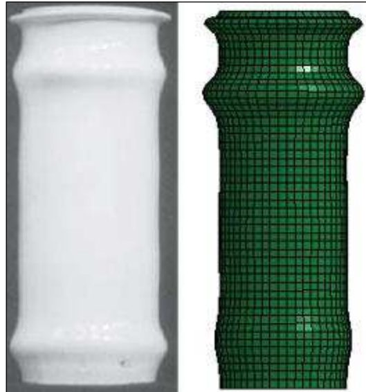
Figure 43 Lu et al. experimental displaced shape (left), Lagrangian fluid model displaced shape (right).
