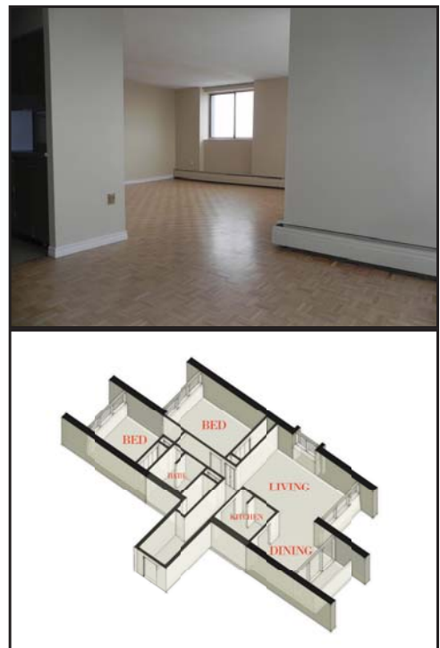
Fig. 59. and 60. Fenwick Place. Above: Photograph of living and dining space in standard apartment. Below: Axonometric projection of standard apartment, showing dual aspect and relation to corridor.
