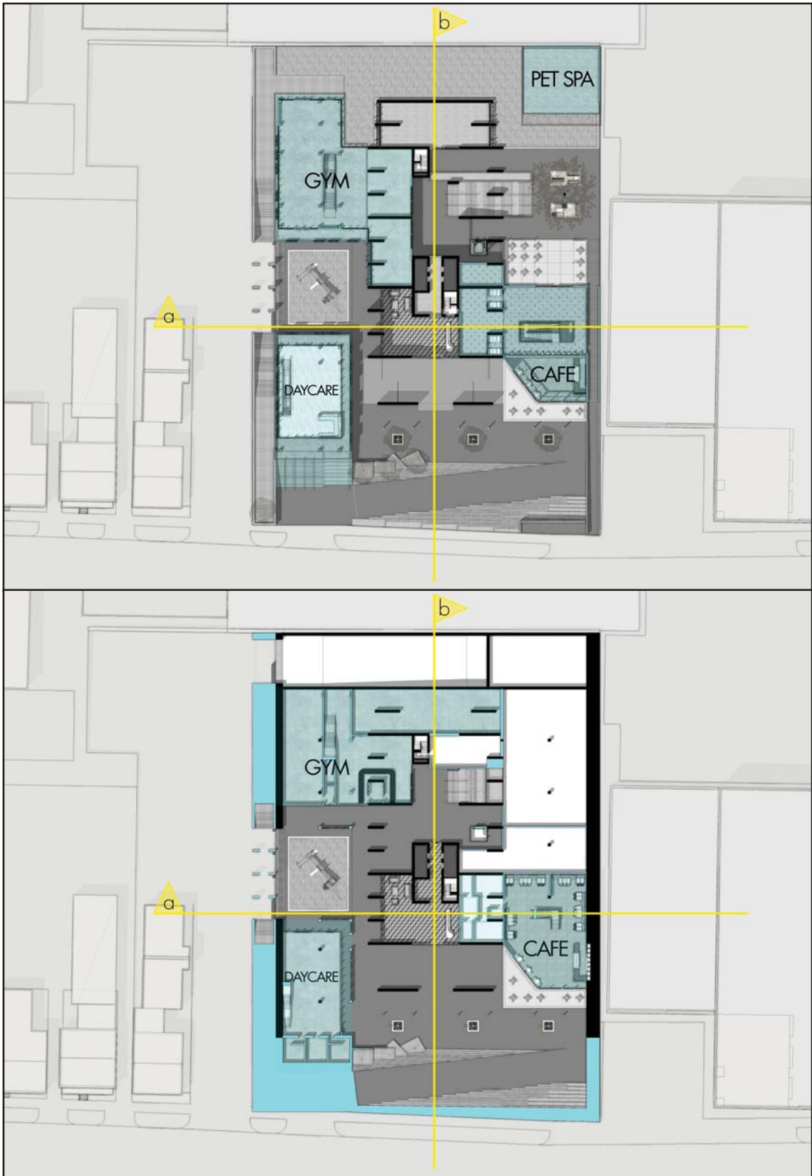
Fig. 140. and 141. Top: Terrace level sectional plan. Bottom: Street level sectional plan. Blue section fill represents new addition, black section fill represents existing structure.
