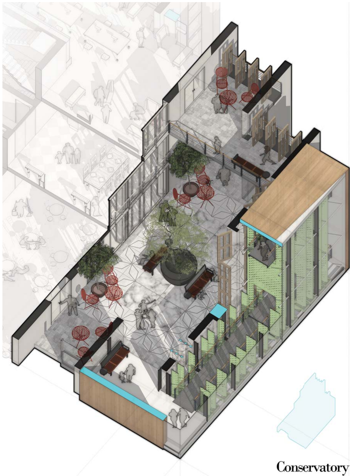
Fig. 162. Axonometric projection of 'graft' intervention. Higher up the tower, this intervention takes advantage of the possibility of cutting into the existing shear walls. Creating larger spaces, this intervention accommodates change not through variation but through atmosphere and an enhanced social environment. Aggregating the activity from the three adjacent floors, and capable of drawing public interest from the plinth, the 'graft' link creates a greater density of social interaction.
