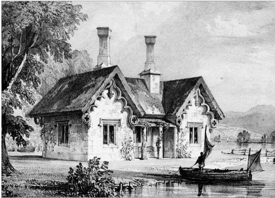
FIG. 15. P.F. ROBINSON'S 1833 DESIGN FOR A "GATEKEEPER'S LODGE," WITH A DEEPLY ORNAMENTED GABLE INCLUDING CARVED GOTHIC BARGEBOARD AND PENDANT. | PUBLISHED IN ROBINSON, 1833, DESIGNS FOR LODGES AND PARK ENTRANCES , PL. V.
