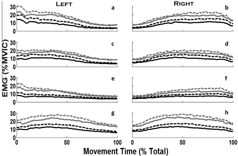
**Fig. 3.** Examples of ensemble average waveforms for specific back sites. Black lines = younger adult group, gray lines = older adult group, solid lines = normal reach, dashed lines = maximum reach. Specific back sites include left (L) and right (R) (a and b) L & RL16 (c and d) L & RL33 (e and f) L & RL48 and (g and h) L & RL52.
