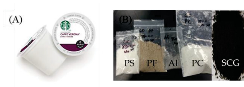
Fig. 5.1. (A) Spent K-Cup (B) ground powder of each spent K-Cup component.
