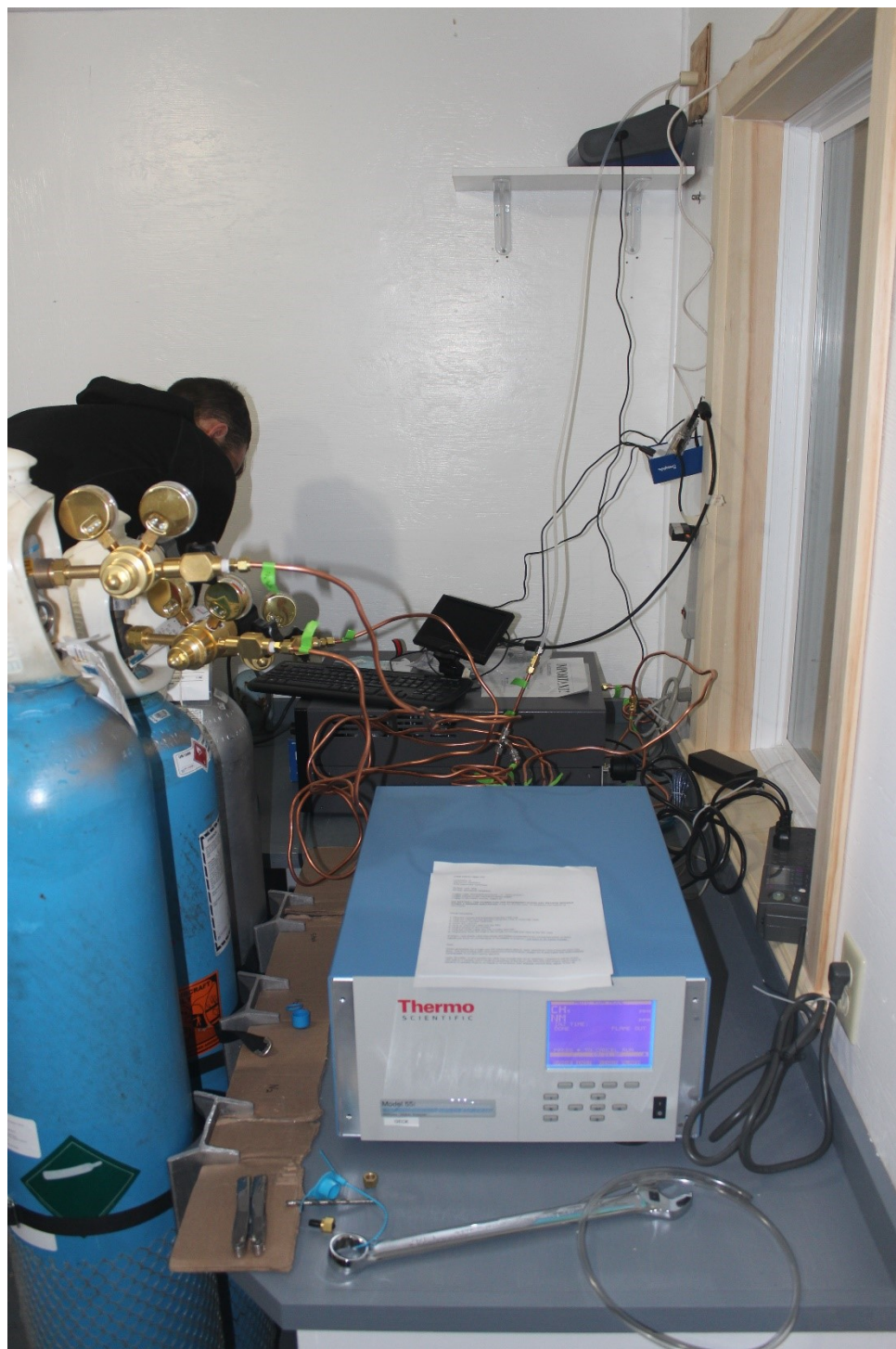
Figure 11. Thermo Scientific 55i set up on Sable Island.
