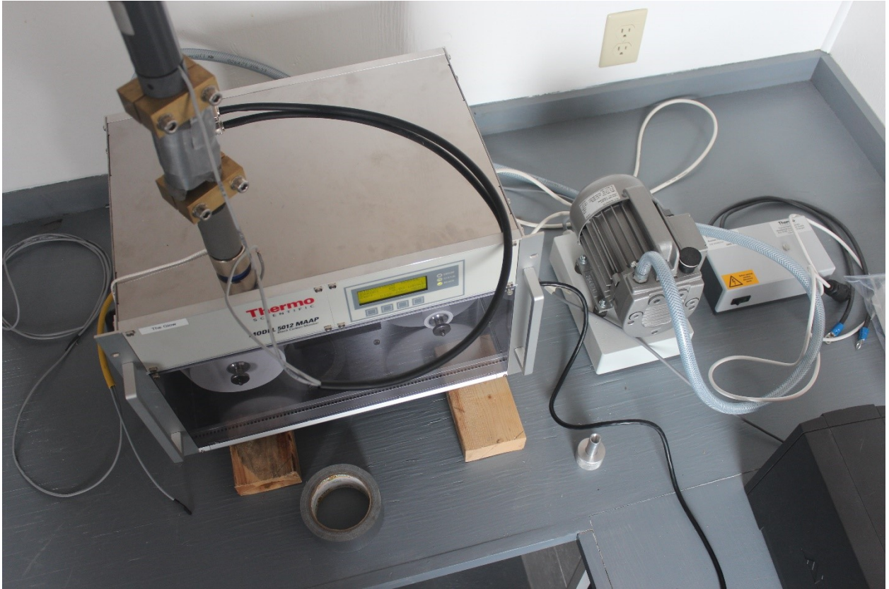
Figure 12. Thermo Scientific 5012 set up on Sable Island.
