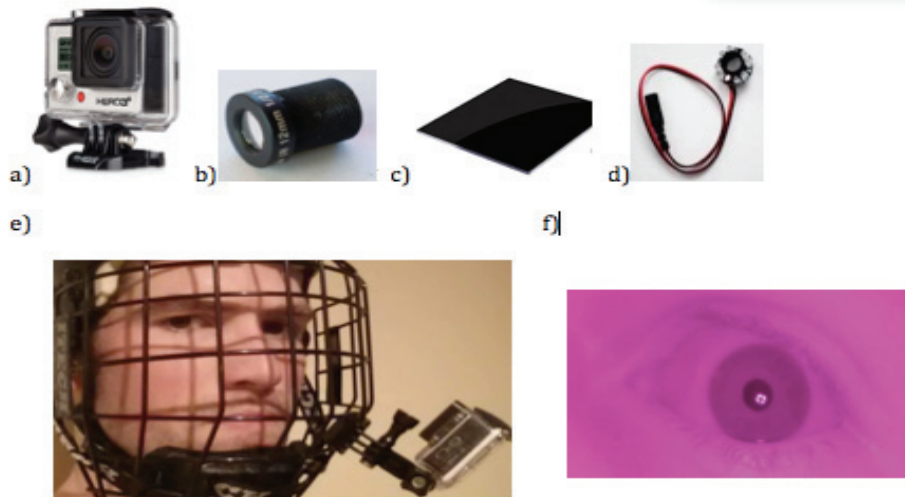
Figure 2. a) GoPro Hero 3+ Black Edition camera. b) 12 mm wide-angle lens. c) Optical cast Infrared long pass filter. d) Infrared LED illuminator. e) Camera attached to cage of helmet. f) Sample image of the eye as seen by the infrared camera. A technical description of the eye-tracking system can be found in Appendix D
