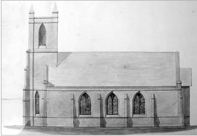
FIG. 30. DETAIL OF AN ARCHITECTURAL DRAWING OF ST. MARK'S ANGLICAN CHURCH FROM 1843; NOTE THE SHALLOW EXTERNAL PROJECTION OF THE CHANCEL. | ANGLICAN DIOCESE OF ONTARIO ARCHIVES, PHOTOGRAPHED BY PAUL CHRISTIANSON, 2008.
