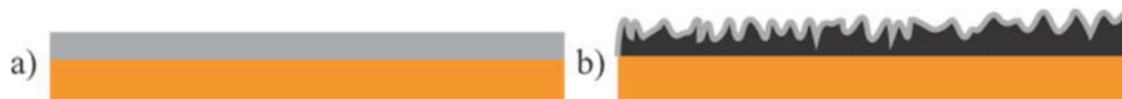
Figure 5.1. Schematic drawing of a lithiated Si thin film (grey) on a Cu substrate (orange) in (a) and on a compliant layer (black) in (b).
