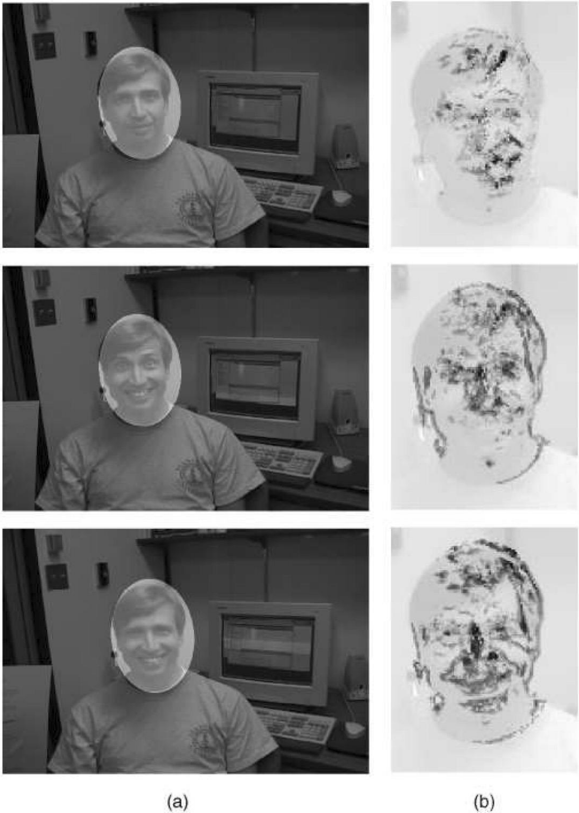
Figure 2.4: Robust online tracking by Jepson et al. [14]. (a) Target object inside an elliptical kernel in successive frames. (b) Stable components obtained from the target patch that are reliable for tracking by applying gradient based technique
