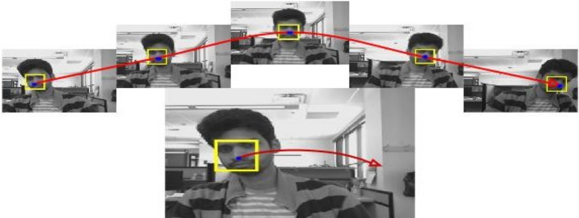
Figure 2.11: The object motion forms a trajectory in a video stream. This spatial and temporal dependency of any image patch provides some structural constraints that aid the semi-supervised learning system in classifying unlabeled data
