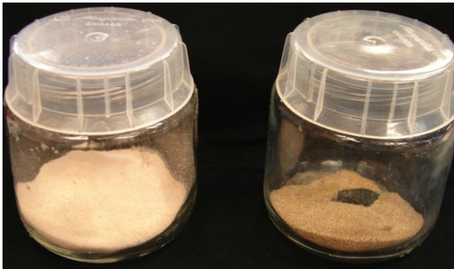
Figure A.1. Lobster shells were grinded, sieved and stored in glass jars at 4 °C. Cooked (left) and fresh (right) lobster shell powder.
