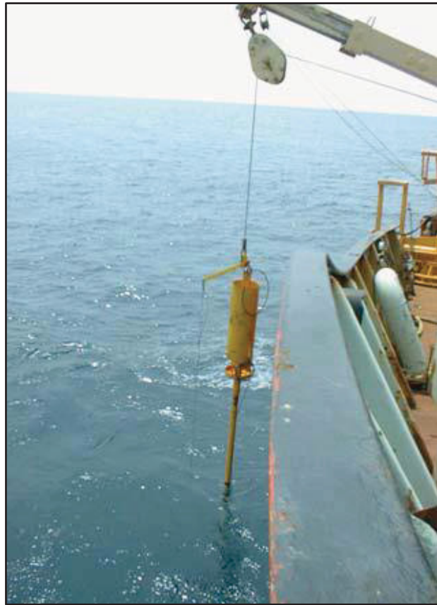
Figure 3.6 Piston Core unit ready for deployment on the CCGS Hudson 2004-030 cruise
