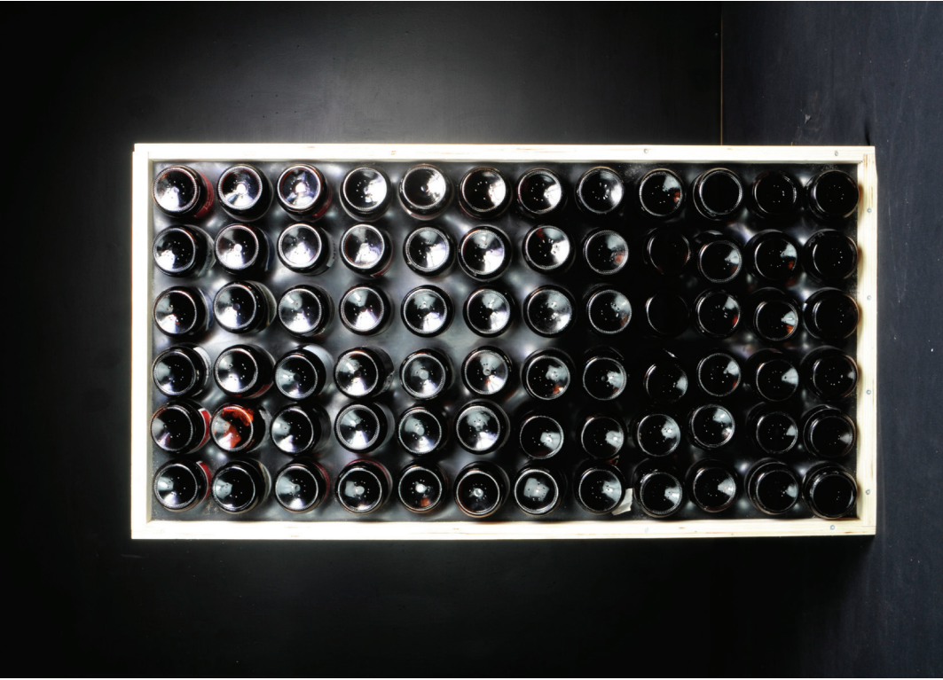
Panel made of wood, rubber, and reused glass beer bottles. The model was created as a 1:1 test of ideas regarding material reuse. When lit from behind, the bottles transmit an amber glow.
