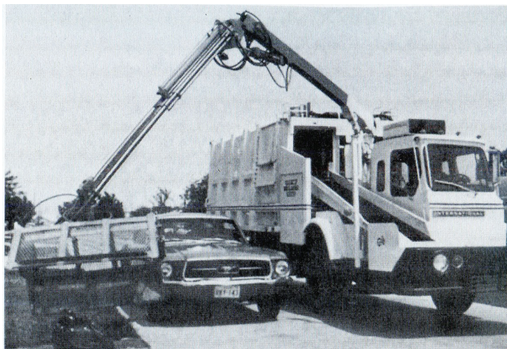
A side-loading municipal refuse truck from '70s had the capability to reach over cars at the curb. Bellaire, Texas (Melosi 1981)
