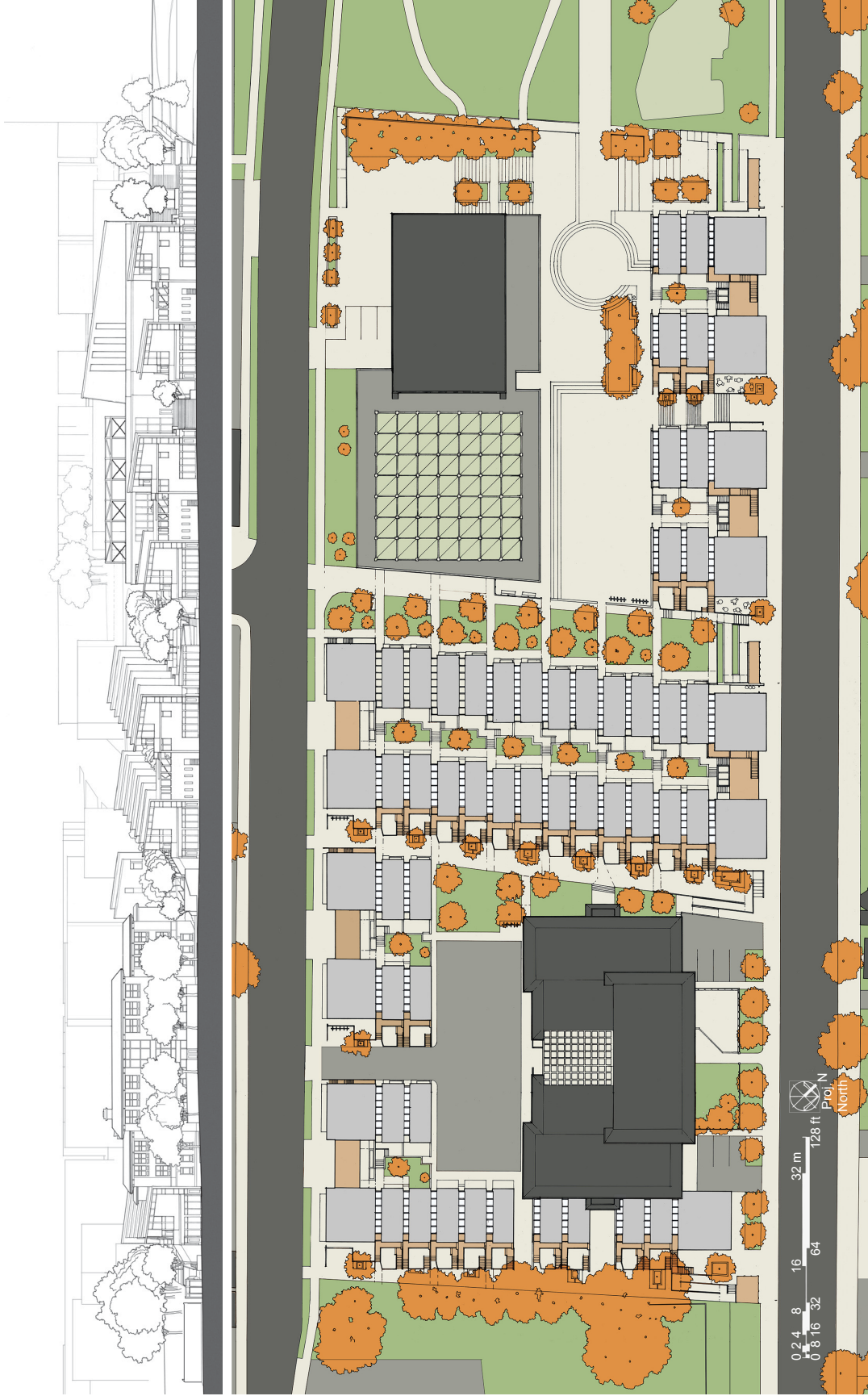
Figure 3.14 Site plan and elevation with a twin row house typology, oriented to the southeast for passive solar warming. The rows stagger to respond to patterns of access in the community, and end units face the street, in order to create an engaged streetscape
