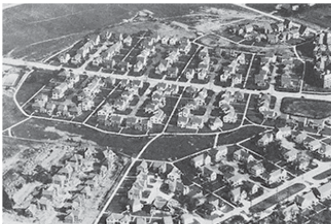
Figure 2.1 Radburn, New Jersey, circa 1929. Shown here is the superblock layout, with a nested system of cul-de-sacs, and pedestrian access paths ( Stein 1951 )
