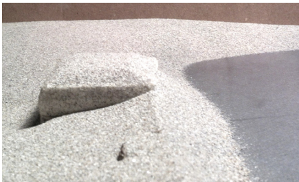
The windward face of the structure accumulates sand.
