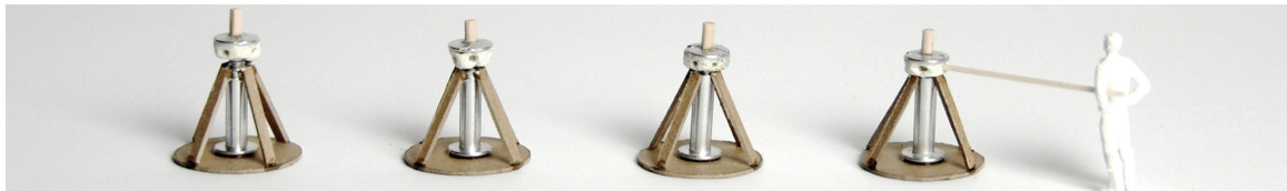
The load on the skis needs to be leveled when not in motion. A screw-jack, hand operated like a capstan on a ship, is integrated into the truss components.
