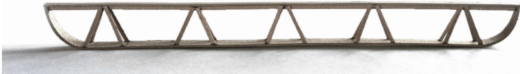
At any point during motion a ski could be partly off the ground, and the load would need to rely on another path, so extra truss segments were added.
