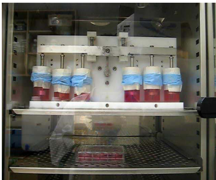
Figure 12 – Inside view of the incubator showing the mechanical stimulation apparatus with samples in place. The upper grip holding the samples was attached to a moving arm that cyclically raised and lowered the bottom grip and weight assembly, loading and unloading the samples. Unloaded samples were maintained in separate wells in a culture plate shown on the bottom shelf.
