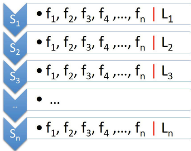
Figure 2.1: An example of data stream. Each flow is shown by “S”, each feature in flow by “f” and respective labels by “L”
