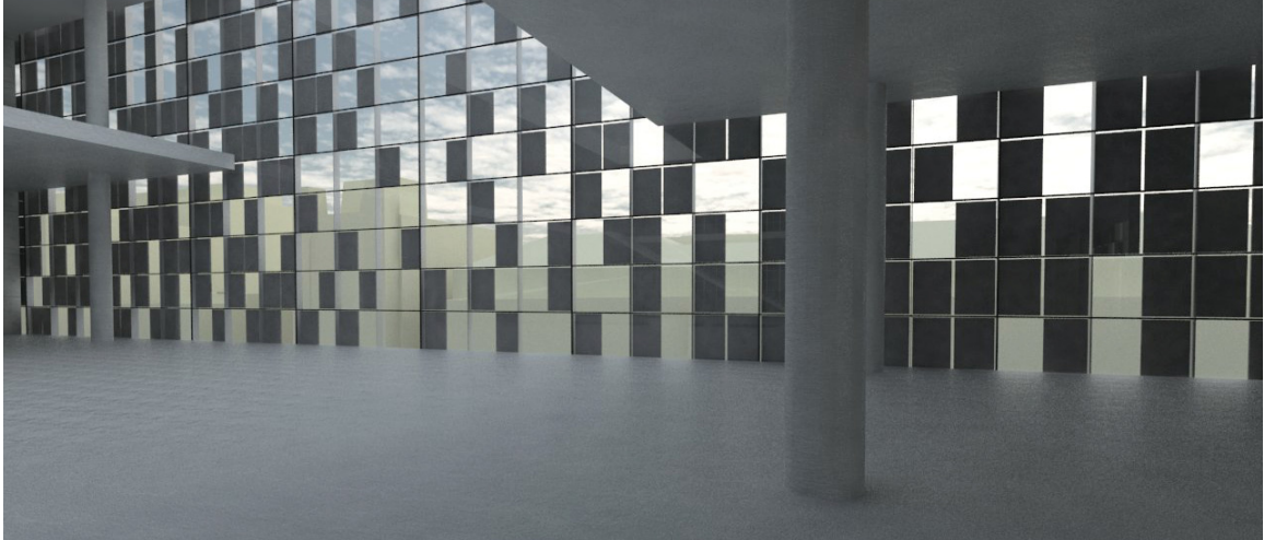
An interior rendering of the hung limestone panel. The panels control the light penetration into the library and acts as an interior finish and lighting feature.
