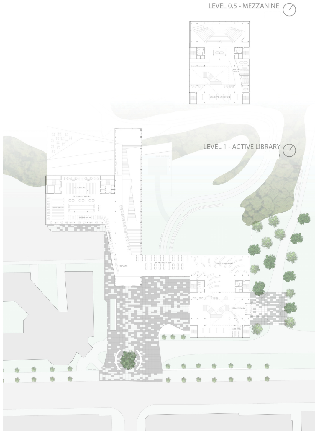
Plan of Level 1: The “indoor street” of the active library linking both library blocks and furnished with activity nodes along its length. The mezzanine contains bookable classrooms and meeting rooms, as well as a large art gallery.
