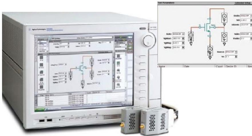
Figure 27: B1500A semiconductor analyzer from Agilent [24]
