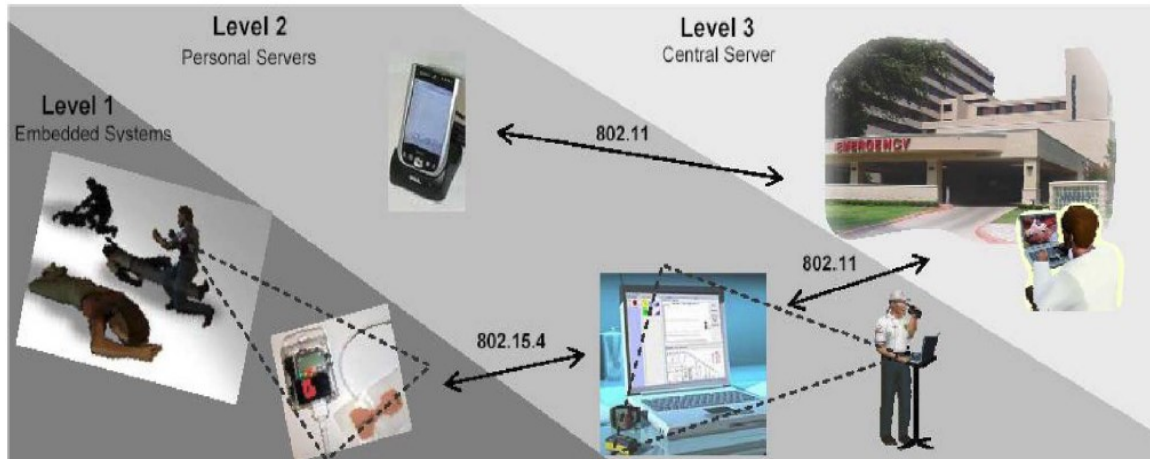
Figure 3-9: Architecture of AID-N system [36]
