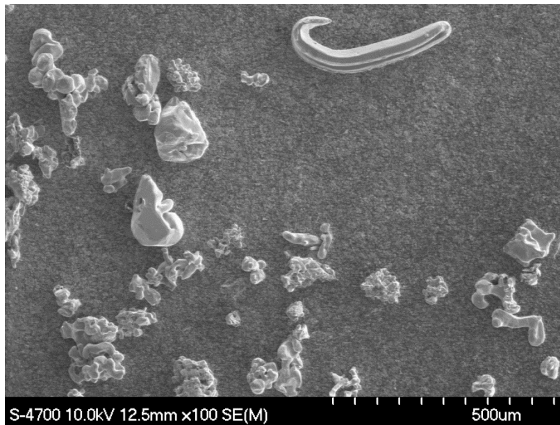
Figure B.4 -100 mesh titanium micrograph-D
