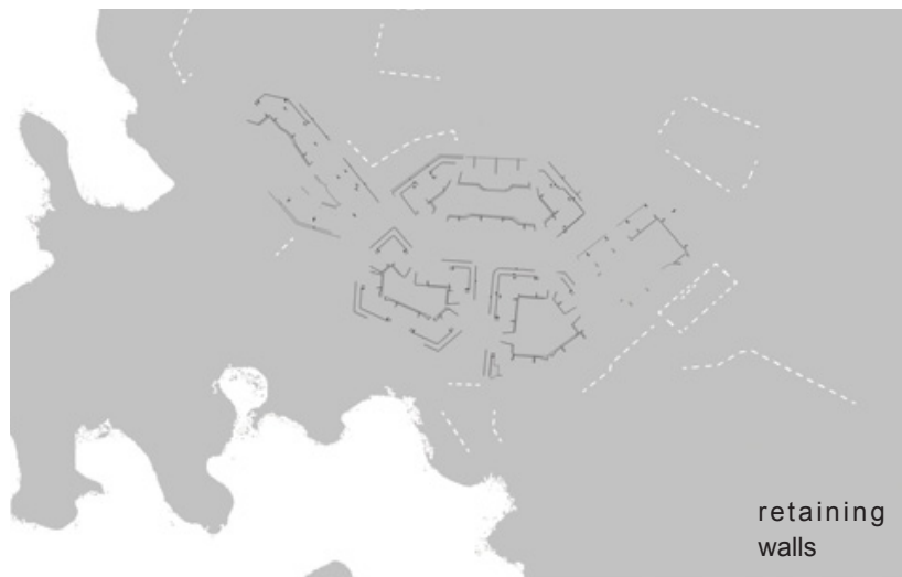
Diagram showing lines (retaining walls) with proposed shown in black and existing in white. Base map from Google Maps.
