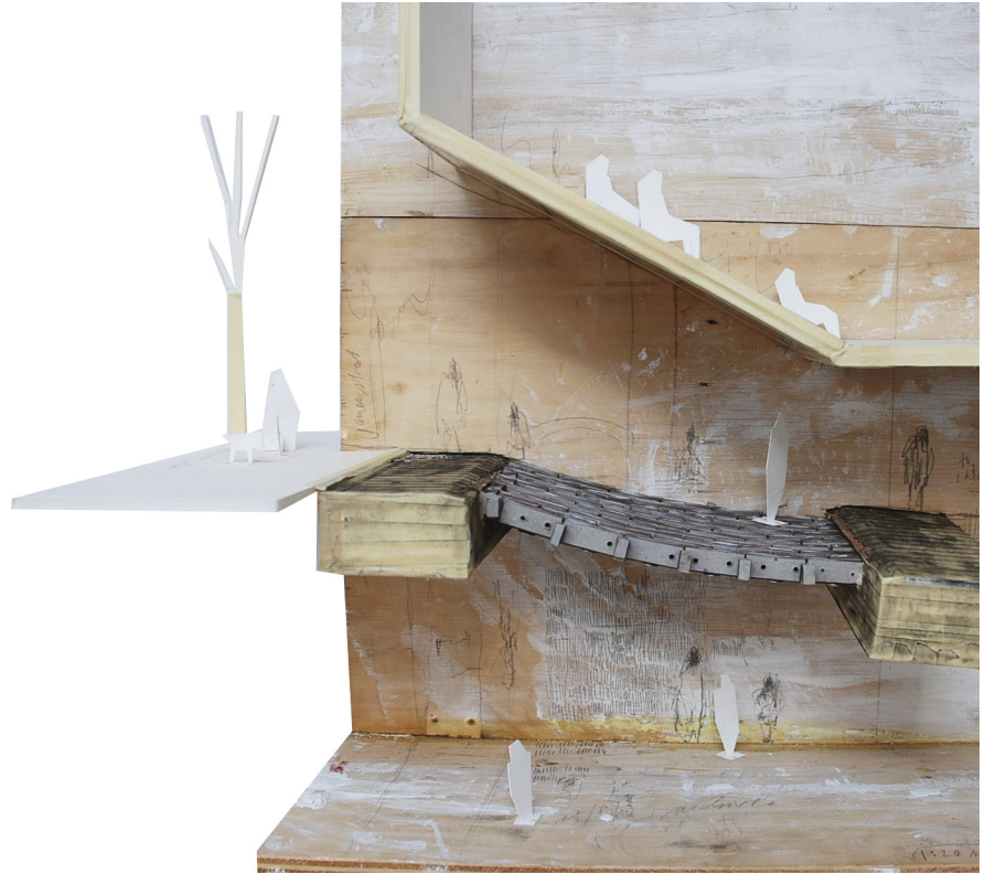
1:25 sectional model of the suspended stone ramp entry.
