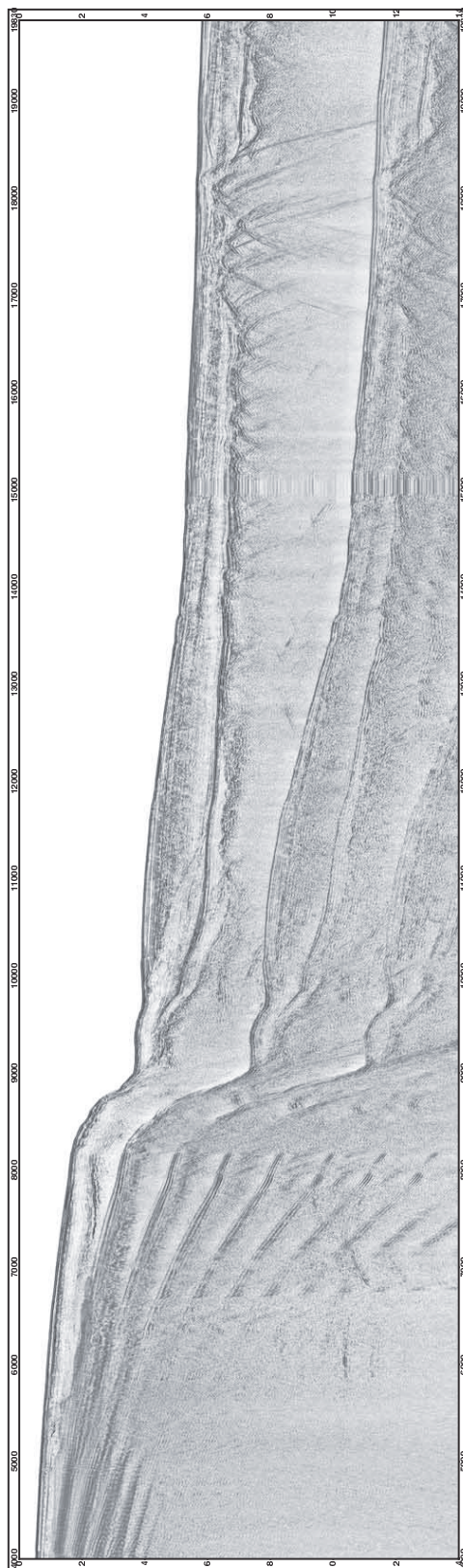
Figure E.12: Stacked section with doubled the shots and new geometry
