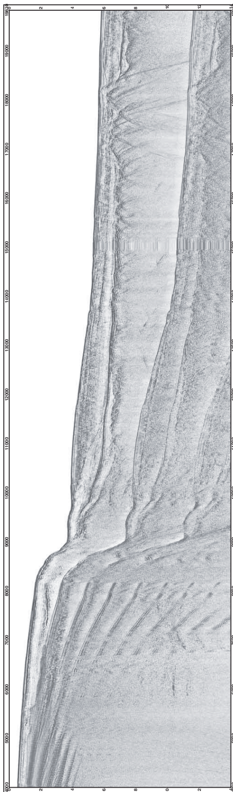
Figure E.13: Stacked section with LIFT applied
