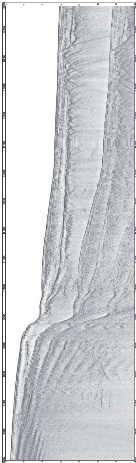
Figure E.14: Stacked section with surface related multiple elimination applied
