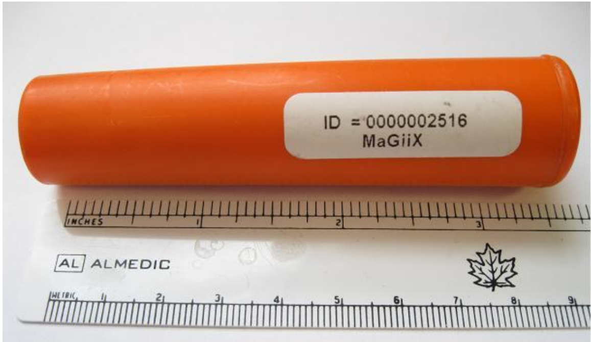
Figure 1: Radio-frequency identification (RFID) transponder bolus containing a thermistor used to monitor reticulo-rumen temperature as part of the Cow Temperature Monitoring System.
