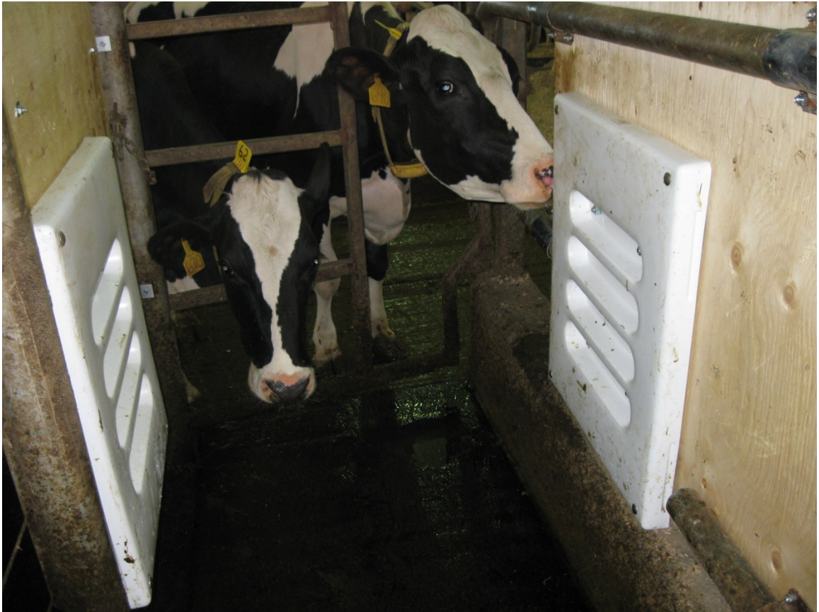
Figure 2: Drive panel (right) and receiver panel (left) for the Cow Temperature Monitoring System set up at the exit ally of the milking parlour at Charles Hill and Sons Farm.
