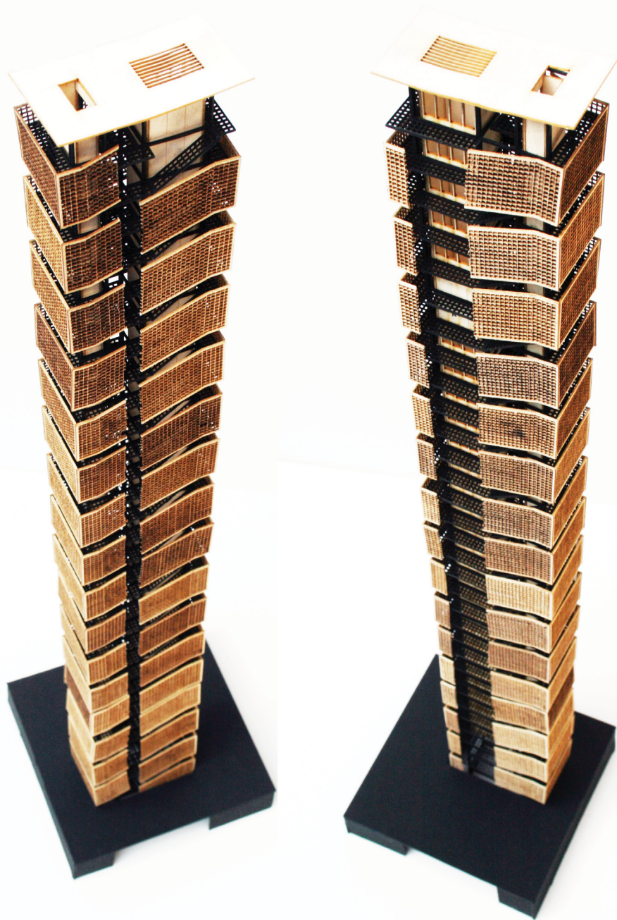
Physical model studies of the proposed solar chimney and vertical circulation shaft within the Robertson headframe.
