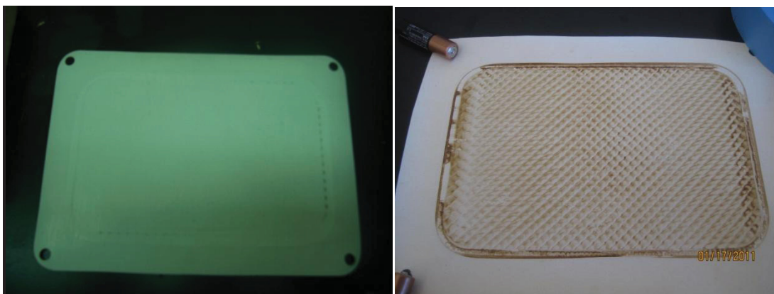
Figure D10 Virgin DK-NF Membrane after 24 hours Compaction with Milli-Q Water (left) and Fouled Membrane with Raw Water from the French River.
