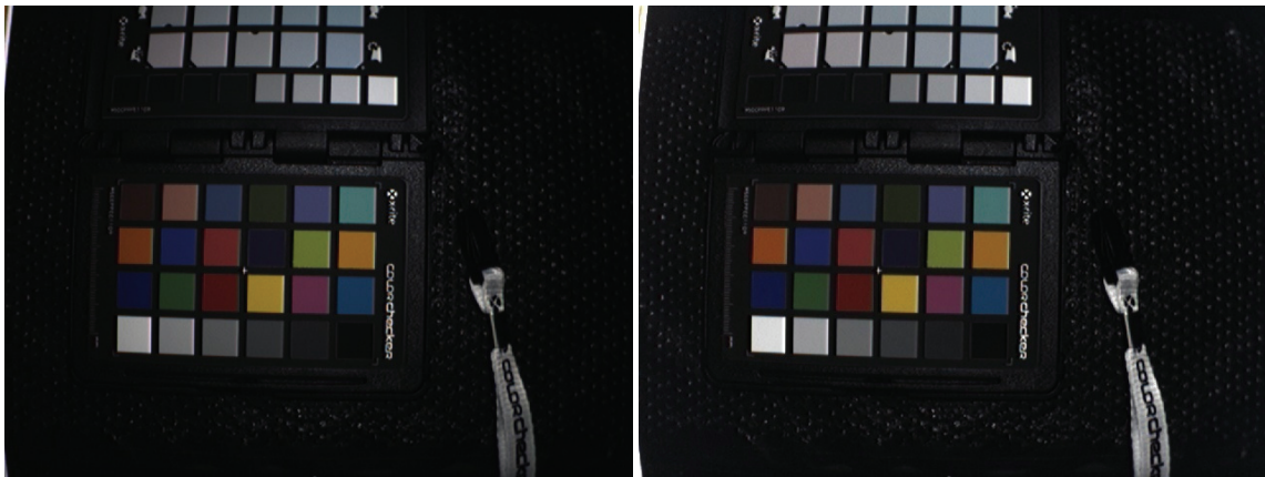
Figure 4.3 Example of Non-uniform illumination (left) and corrected uniform illumination (right) using the colorchecker passport
