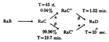
Radium C" was isolated by Hahn and Meitner<sup>1</sup> by recoil and was shown to decay with a period of 1.32 minutes giving out  $\beta$  rays. The emission of  $\alpha$  rays from RaC has never been demonstrated experimentally. From the branching ratio it can be surmised that the period of these RaC atoms is about 45 days and from the Geiger-Nuttall relationship their  $\alpha$  particle range should be about 3.6 cms.
