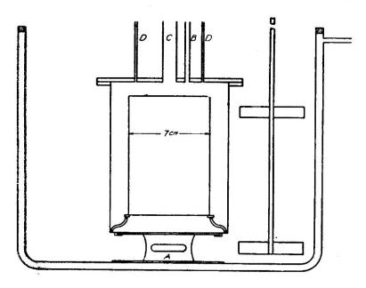
The apparatus shown in the diagram, was constructed by Mr. G. Sandos to whom our thanks are due. It is essentially the same as the ordinary calorimeter with four stirrers, but the outer chamber was a copper Dewar flask, 15 cm. wide and 20 cm. deep, connected to a pump which maintained a good vacuum (0.001 mm).
