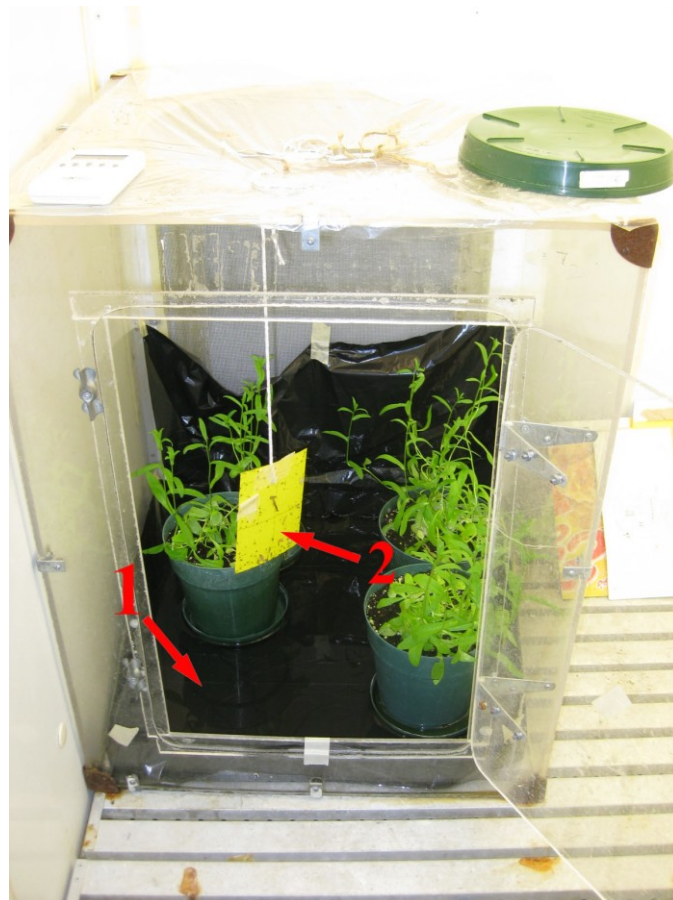
Figure 2.2: The cage used for maintaining inoculated host plants (RH ranges from 70% - 80% inside). 1. A thin layer of water; 2. Insect sticker.
