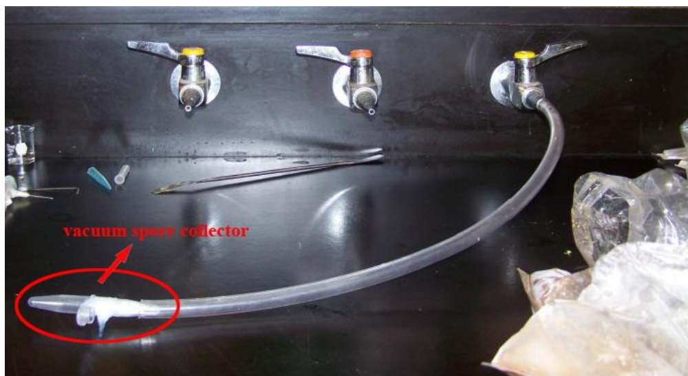
Figure 2.1: The vacuum spore collector used for conidia collection
