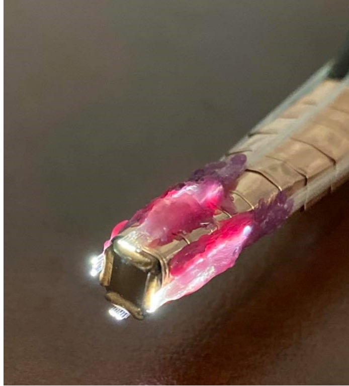
Figure 5.11: Photoacoustic fiber optic cables temporarily fixed to the 30 MHz 3D phased array ultrasound transducer using wax.
