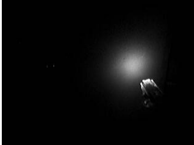
Figure 5.3: Illumination pattern at 12mm away from the endoscope tip.
