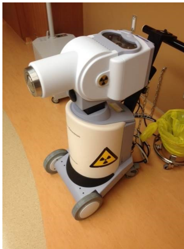
Figure 11 - MicroSelectron remote afterloader, made by Elekta. Photo taken from the Nova Scotia Cancer Centre.
