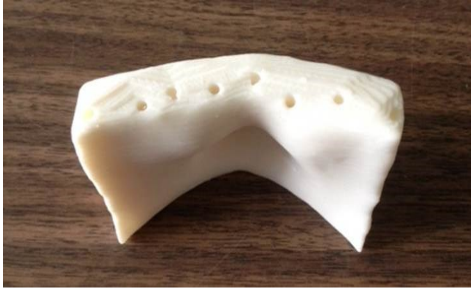
Figure 26 – Programmed 3D printed applicator showing catheter tunnels for placement of radiation source.
