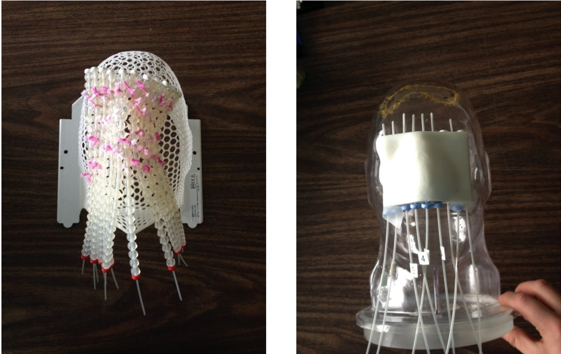
Figure 28 – Head phantom fitted with Left: FF applicator. Right: 3D printed applicator.
